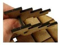
Insert [B14] into the hole on [B1] and [B2]. Make sure that [B14] does not go beyond either side.
